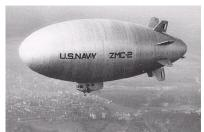
The **ZMC-2** (Zeppelin Metal Clad 200,000 cubic foot capacity) was the only successfully operated metal-skinned airship ever built. Constructed at Naval Air Station Grosse Ile by The Aircraft Development Corporation of Detroit, the **ZMC-2** was operated by the U.S. Navy at Lakehurst, New Jersey from 1929 until its scrapping in 1941. While at Lakehurst it completed 752 flights, and logged 2265 hours of flight time
