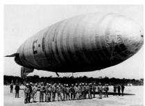
The **E class** of US Navy blimps comprised a single airship, built during World War I by Goodyear as one of a group of three small blimps offered to the US government. Two were purchased for the US Navy and one for the US Army and used primarily as training airships. The Navy blimps were designated **E-1**, **F-1**, and the Army airship **A-1**. These airships had identical envelopes but different cars. First flight at Pensacola in December of 1918, retired in 1924; one built.
