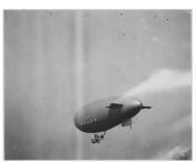
The **D class blimp** was a patrol airship used by the US Navy in the early 1920s. The D-type blimps were slightly larger than the **C-type** and had many detail improvements. The Navy continued the practice of dividing the envelope production between Goodyear and Goodrich. The control cars were manufactured by the Naval Aircraft Factory. First flight 13 July 1920 at Wingfoot Lake, Ohio, retired in 1924, 6 built.
