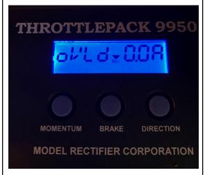
The blue display shows the voltage and current supplied to the track. For our standard operation, that is in the general area of 14v and 0.5A. If there is a short circuit, the display changes to "oVLd 0.0A" and the train won't run. Short circuits can be caused by metal objects dropped across the rails and by derailments.
