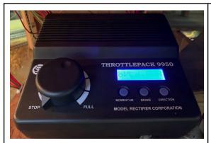
The speed knob on the base station should be turned all the way to the left until it hits the end of motion near the "Stop" label. If this knob is turned up, the walk-around speed control may be erratic.
